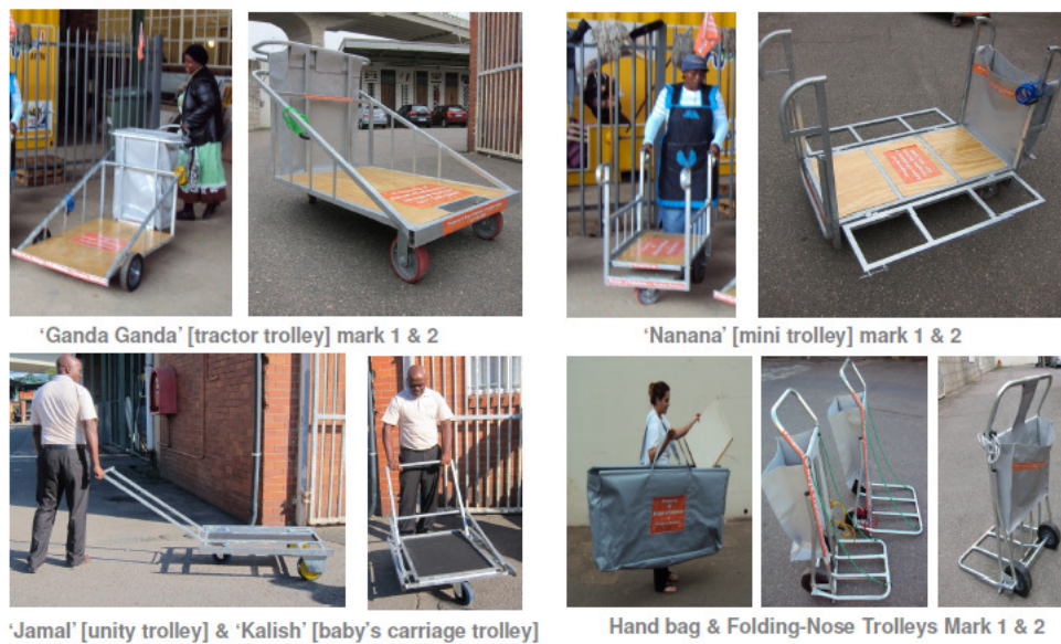
Figure 4: Various trolley proto-types tested for the project to address the challenge of conveyance of waste recyclables
